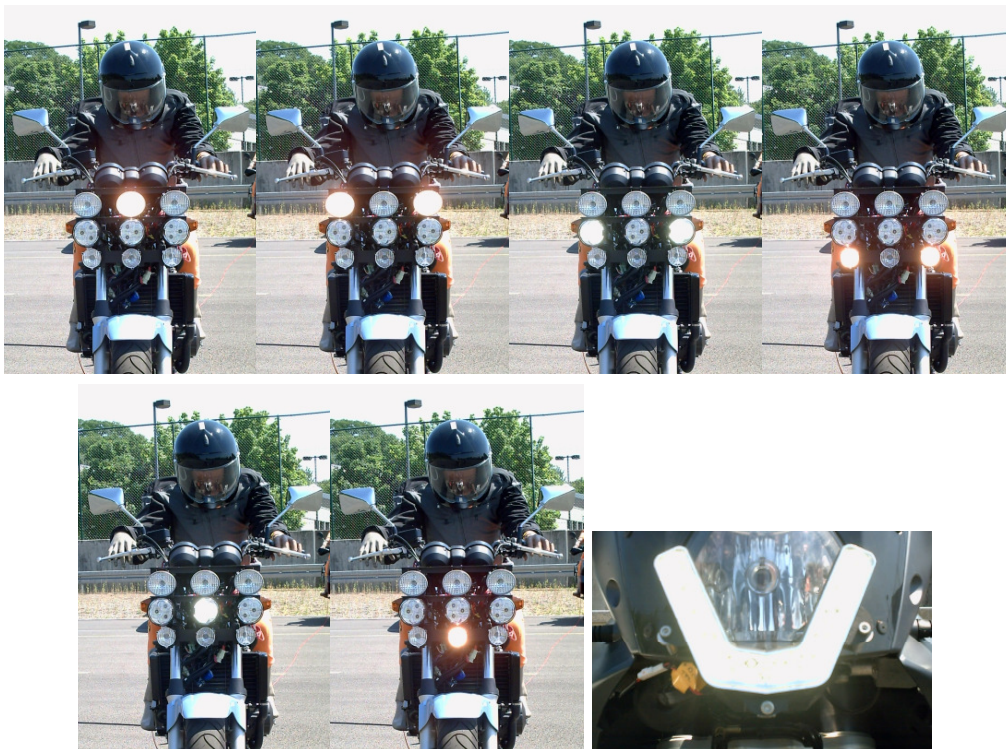
Figure 2: Experimental vehicle equipped with different dedicated daytime running lamps (signal pattern A-G of test series 2)
